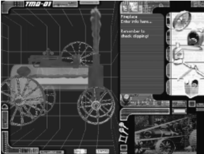
**Figure 4.** A PC-based model developed for the Museum of Technology, Delft. It is aimed at young learners to show the basic principles of a 'locomobile'. Five main elements are dragged and put together into the workspace. When the assembly is correct, the Locomobile starts to operate and a dialogue then explains the principles of the steam Locomobile.
