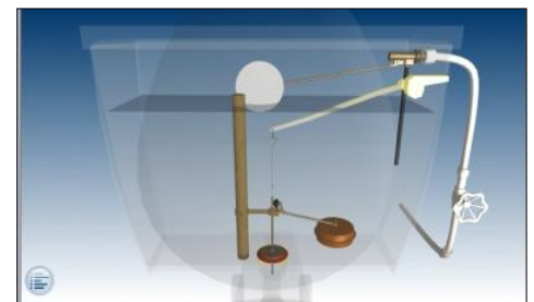
Water conservation: simple repairs to a toilet cistern
